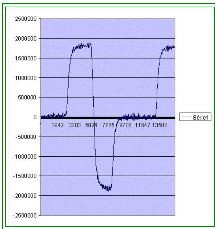
**FIG. 15 : 32 Hz sampling during 8 minutes, with rotation of one or two revolutions of the gravimeter vernier. Each time the vernier is turned, we observe a transitional period of at least one-minute to reach the equilibrium position.**
