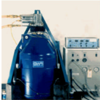
remote Controlled Superconducting Gravimeter. This model generates its own LHe.
